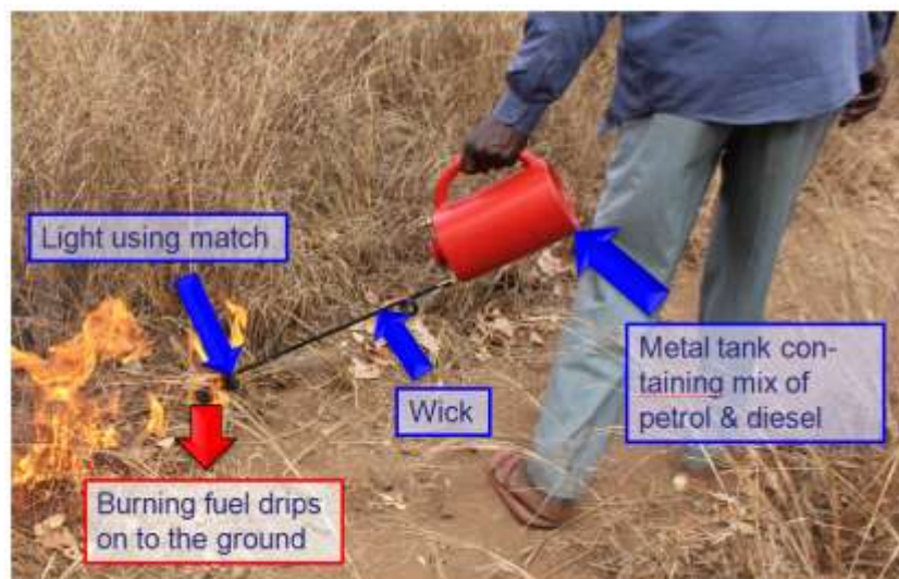
Figure 34. A drip torch and its use.
